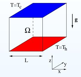
$\mathbf{Ra} = g\beta L^{3}\Delta T/\alpha\nu$  $\mathbf{Pr} = \nu/\alpha$  $\beta \text{ thermal expansion}$  $\nu \text{ kinematic viscosity}$  $\alpha \text{ thermal diffusivity}$  $\Delta T = T_{h} - T_{c}$
